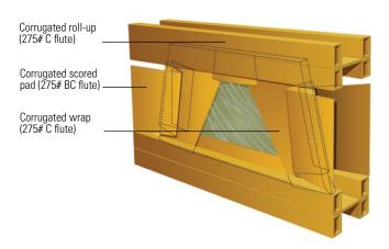
This design helps protect windshields from shock and/or torque during transit. The wrap converts a non-rigid part into a rigid surface so it can be cushioned and braced off of the corrugated wrap.
