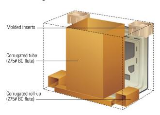
This design helps protect the trunk pack from external forces. Molded inserts are used to create air cells and brace the trunk lid.
