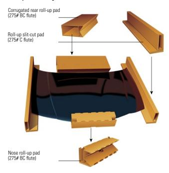
With this design, you center the nose and rear roll-up pads and staple them to the inner flaps of the end-loaded full-overlap shipping container. Place the hood in the container followed by roll-up slit-cut pads. Close and tape.
